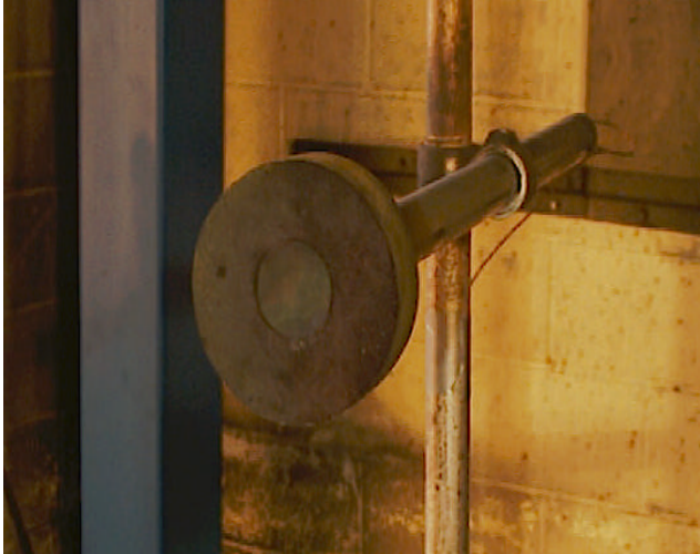
FIGURE 1. Copper Calorimeter On Test Stand
