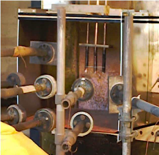
FIGURE 4. Test Setup No. 3 3 Phase Flat Electrodes In Box
