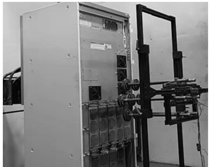
Fig. 9 Placement of slug calorimeters
