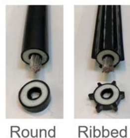
Fig 15. Semi-conductive Shielded Skin Effect Insulated Conductors
