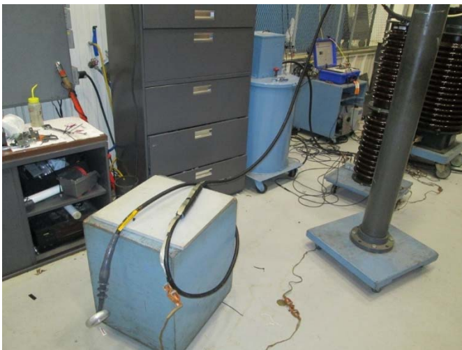
Fig 13. Partial discharge test setup for skin effect insulated conductor splice joint assembly
