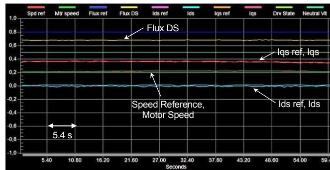
Fig. 11 (b) Drive variables under light load at 52Hz. Speed Reference and Motor Speed signals are offset by -0.80.
