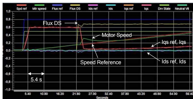
Fig. 10 Drive variables during motor start in i/f mode and transition to sensorless vector control
