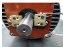
Fig. 16 Motor with shaft grounding brush and shaft voltage measurement brush
