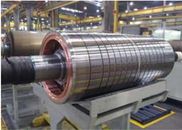
Fig.10 Squirrel cage rotor with non-magnetic retaining ring.
