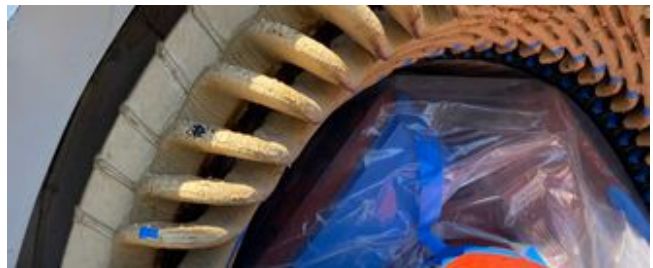
Fig. 6 Wrap Rotor for Protection
